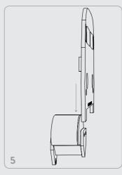
5. Take the front of the lamp and slide it down on the front area on the lamp socket. Connect the LED driver to the lamp and then to the supply
