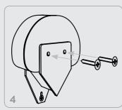
4. Fasten the plastic cover to the lamp socket with two of the included screws
