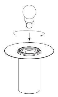
Once the bulb is in place, place the lampshade onto the lamp base, aligning the grooves in the metal ring in the shade with the bayonet fitting on the lamp base. Turn clockwise and tighten securely.
