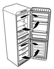
The inner ventilation system cools food more rapidly and keeps refrigeration homogeneous inside the appliance.
