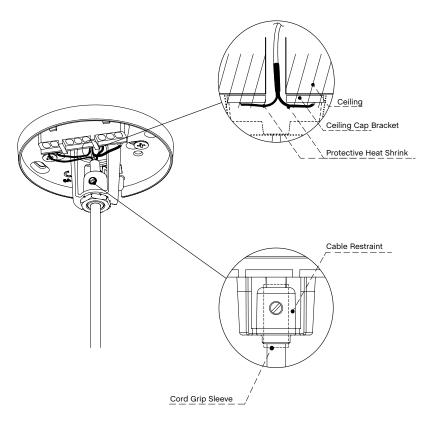
If utilising the mouse hole cable exit, please note the internal cable restraint and integrated cable clamp. The cable clamp tab can be removed and cut to the desired length to suit length to suit the cable thickness used, if this is longer than what is already provided.
