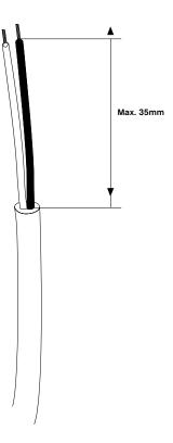
There is a 5mm wire strip guide provided on the internal cover, as shown below. Strip 5mm of exposed wire carefully, ensuring both layers of insulation are intact and not damaged.
