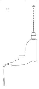
Trim the cable to the desired length, leaving 35mm of basic single insulation exposed for wiring.
