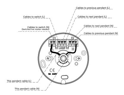
Check to ensure that the protective heat shrink, the cable restraints and cord grip sleeve are still in place after fitting all wires. Check that all of the Live, Neutral and Ground connections are securely connected before switching the power back on at the mains. Ensure there are no loose cables or exposed bare wires and that the clear ceiling bracket is securely fixed to the ceiling.
