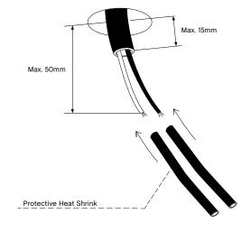
A heat gun can be used to shrink and fix this protective insulation in place, as shown below.
