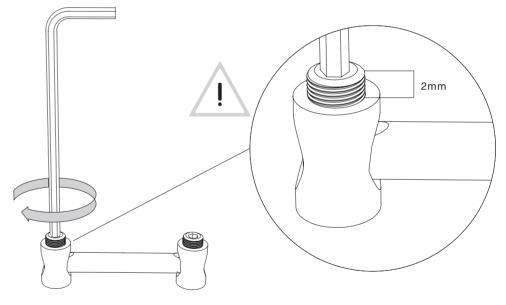
3. Tighten the E parts completely.
