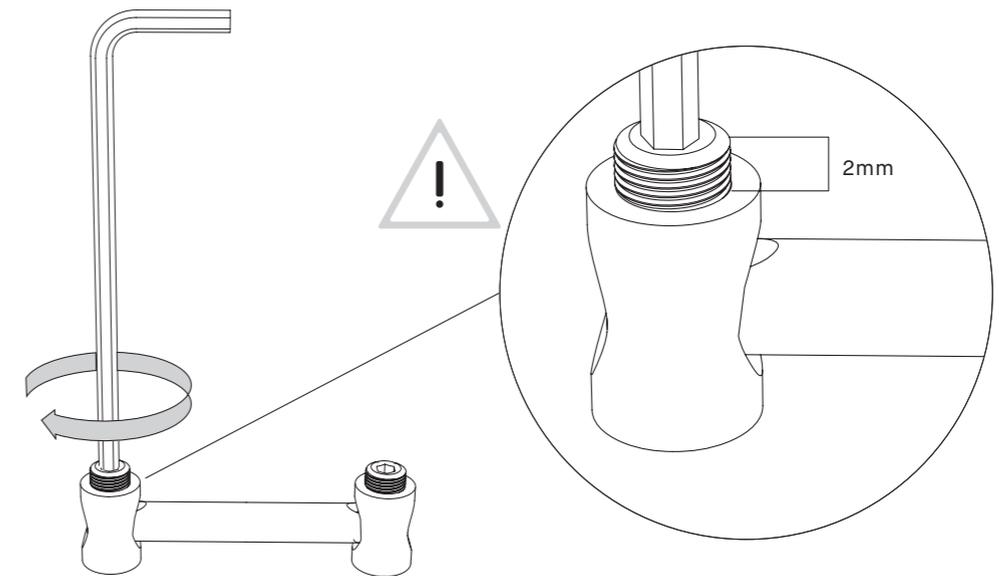
3. Tighten the E parts completely.
