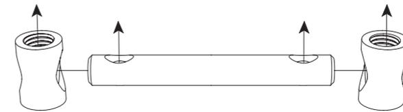
2. Insert the E parts into the C parts and screw each of them half way in a first phase, to make sure they both fit the D parts tapered holes.
