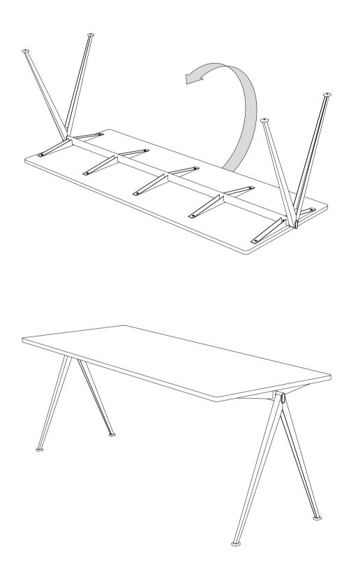
Make sure the table is level and then tighten the C parts completely.
