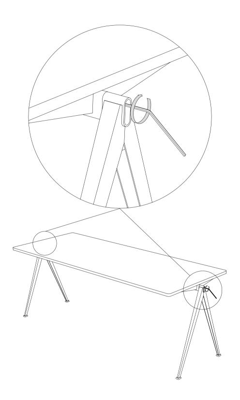
Make sure the table is level and then tighten the D parts completely.
