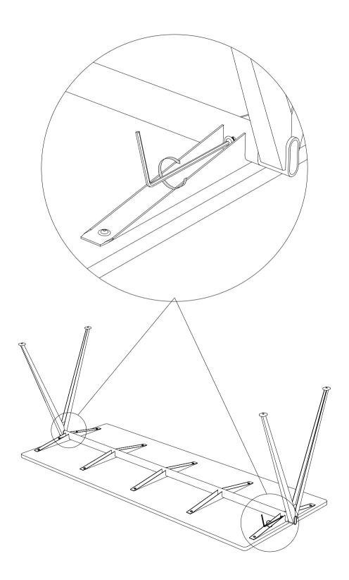
Secure A to B by slightly tightening the C parts. Do not tighten completely at this stage.
