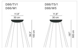
NOTE: The final shape of the luminaire may vary according to the length of the suspension cables.
