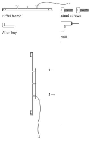
first screw the top hole, than continue with the bottom hole
