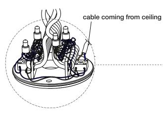
Attach the single blue cables to the terminals and tighten the screws.
