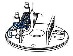
Connect all blue cables using the connecting device, making sure that all cables are touching each other inside the connecting device.
