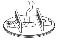
Insert the cords through the canopy holes and cut the cords at the right length, leaving out the inside cables. Leave approx. 5 cm. for installation.
