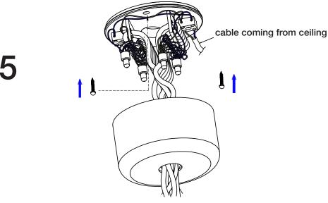
Attach the terminal to the ceiling using raw plugs and screws.
